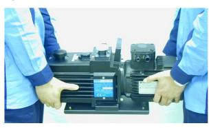
Fig. 3 Transportation method of the oil sealed rotary vacuum pump
